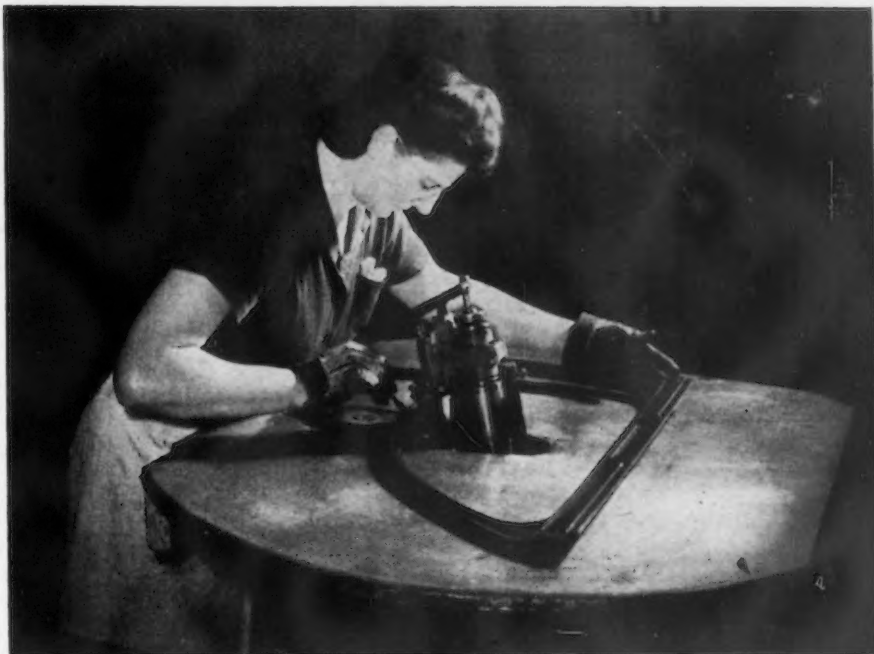
FIG. 4—A graining machine which permits application of the grain to curved surfaces.
